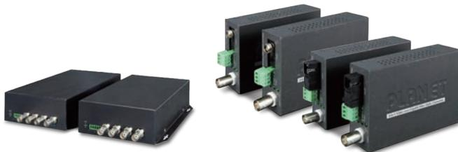
PLANET has developed the video over Gigabit fiber media converter kit, VF-101G/102G/106G/402-KIT, which is ideal for extending the distance and signal conversion by transmitting the AHD/CVI/TVI/CVBS video and data over the fiber-optic cable.
